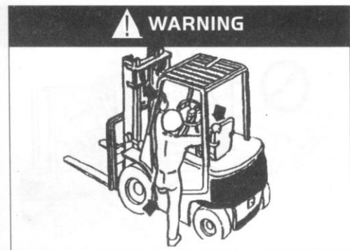
Hold the handrail during on-boarding
