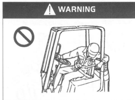
Keep the body under the overhead guard!
