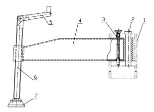
1 Chassis2 Axle Pin3 Aligning Pin4 Turning Leg5 Handle6 Supporting Bolt
