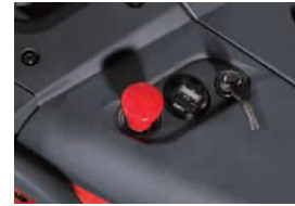
Key-switch, emergency switch and battery discharge indicator.
