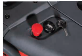
Key-switch, emergency switch and battery discharge indicator.
