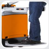
2. Aluminium, suspended platform is spacious. Together with the cushioned, wide sidebars placed in a right height they offer excellent support and drive comfort.
